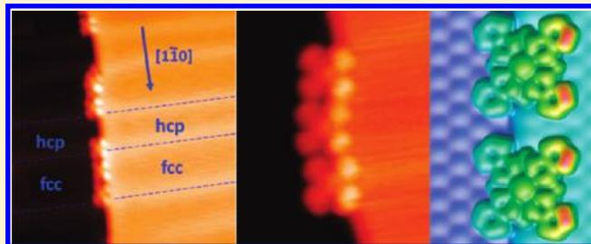
The exact adsorption site and configuration of the FePc molecule as well as the simulated STM images are obtained on the basis of DFT calculations, which is in good agreement with experimental observations.
